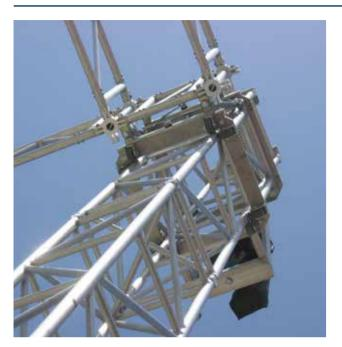
The Maxitower 52HD is a high performance, high capacity tower for your large and demanding projects. Made from EN AW 6082 T6 aluminium, it has the same dimensions as the Maxitower 52 but features Ø 60 x 5 mm main chords for achieving higher load capacities. Thanks to these unchanged dimensions, it's compatible with the standard Maxitower 52 sleeve block.
