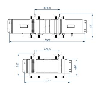
The HiPe Q76 is not just a tower, but a coordinated system of modules and accessories to stabilize it on the ground, with both metric modularity and full compatibility with the Layher scaffolding standard.
